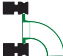
*clamping and rotating of a flange with elbow*
